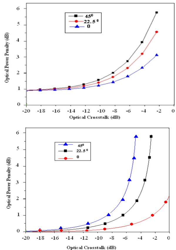
Fig.6 optical power penalties (a) for in-band Crosstalk (b) for out-of-band cross talk (simulation)
