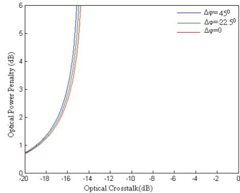
Fig. 3 Optical power penalties for in-band crosstalk for 8-QAM modulation
