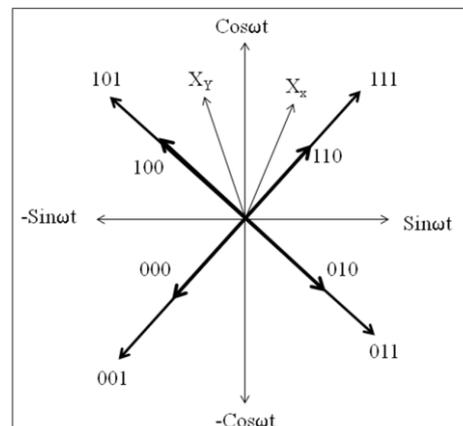
Fig. 2 Signal constellation showing 8-QAM signal and offset crosstalk signal
