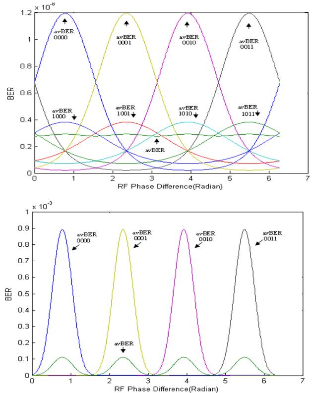
Fig. 5 BER versus RF phase difference (a) for  $-30$  dB crosstalk and (b) for  $-10$  dB in-band crosstalk
