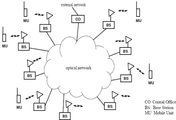
Fig. 1 Fibre-radio network comprising optical fiber and wireless networks.
