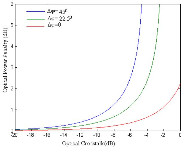
Fig. 4 Optical power penalties for out-of-band crosstalk for 8- QAM modulation
